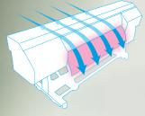
The air flow inside the printer has been redesigned for faster ink drying. The air flow system brings air from the rear of the printer and then blows it along the front cover out of the printer. This air flow coupled with a large heater makes it possible to quickly dry even low odor inks.
