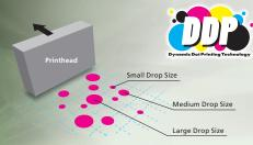
Dynamic Dot Printing Technology controls and optimizes dot size to produce rich, bold and glossy colors with fine details. DDP also creates high density printing without any loss in speed, giving the ColorPainter M-64s backlit film capabilities.
