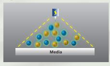
Static electricity on print media is one of the major factors that cause printing defects. The built-in on-carriage ionizer neutralizes static electricity and eliminates static related print issues, even in a low humidity environment.
